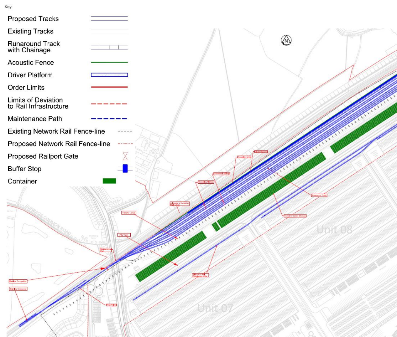
Fig 59. Western Arrangement of Main Reception sidings, intermodal sidings and container storage. Document Reference 2.25
