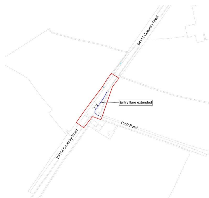
Fig 55. Proposed Works to Coventry Road / Croft Road junction east of Croft (Document Reference 6.3.3.3)
