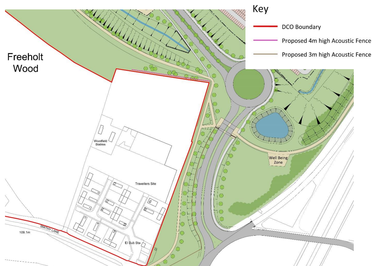
Fig. 64 Proposed Noise Barriers around Aston Firs (Document Reference 6.3.10.10)
